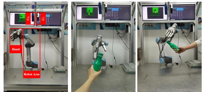
Fig. 10: The hardware setup of our handover system. Key hardware are marked in four red boxes. “ $C_H$ ” denotes Ensenso N35 for high precision camera, “ $C_L$ ” denotes Azure Kinect for low precision camera. Two cameras capture the scene from the backside at a 45-degree viewpoint. “Hand” denotes HIT-DLR II anthropomorphic robot hand. “Robot Arm” denotes UR5 robot arm. The handover experiments are conducted from frontal and lateral two delivering positions.
